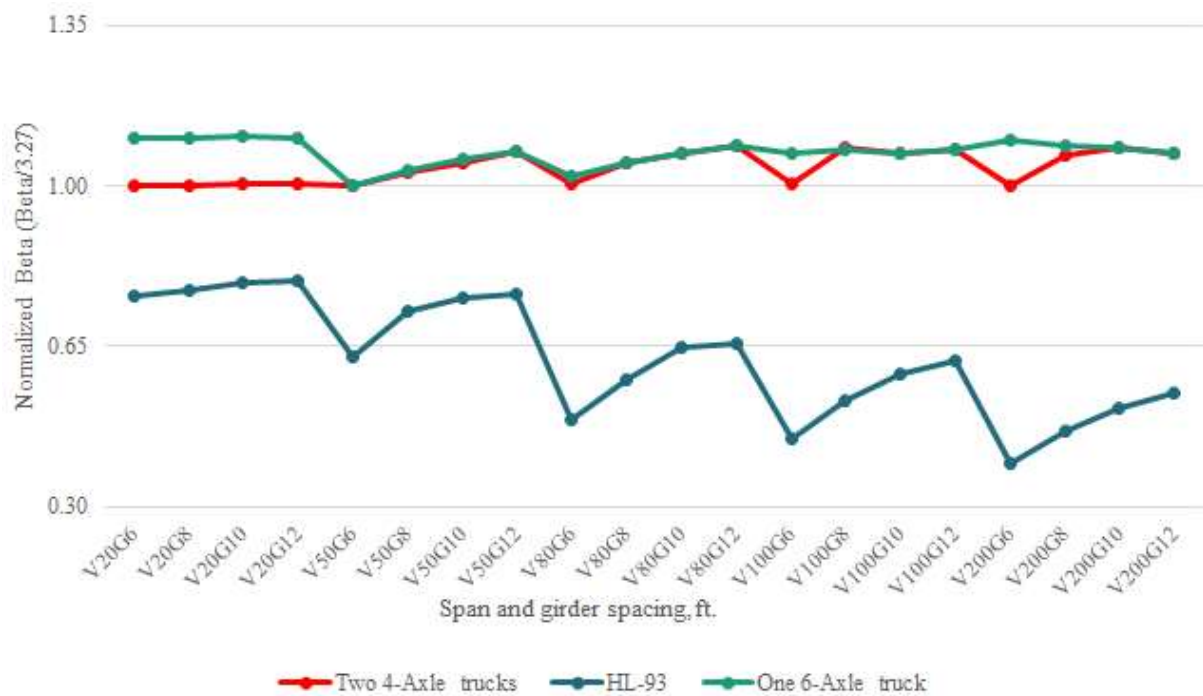
Figure 7.12 – Comparison of 6-axle truck, HL93 and two 4-axle trucks
